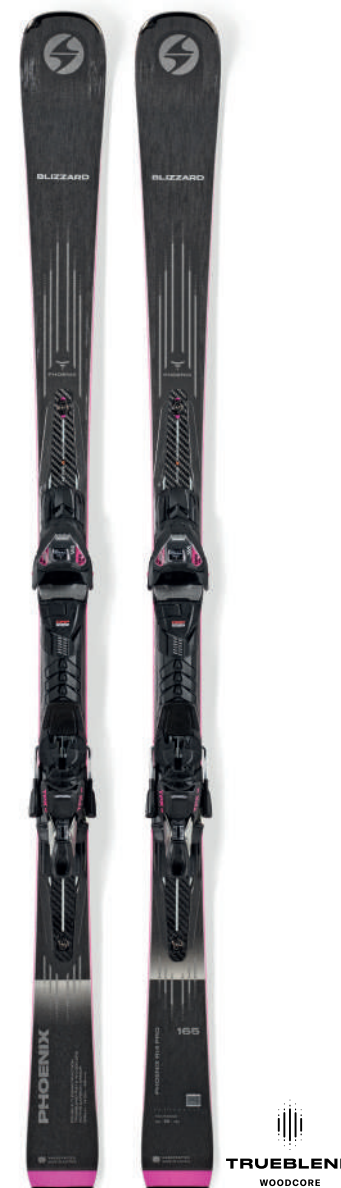
PHOENIX R14 PRO + TPX12 DEMO W COD: 8A1045 00 001 Lengths (cm) / Radius (m): 155/11.5, 160/12.5, 165/14, 170/14.5, 175/15 Sidecut: 121-70-102 mm (165) Plate: FDT Race Plate Binding: TPX12 DEMO W DIN: 4-12 Construction: Sandwich Compound Sidewall (2Ti), Trueblend Piste, Active Carbon Armor, Duramax Construction Rocker: Full Camber Core + Key materials: Trueblend Piste, Poplar - Beech Factory base bevel: 0.9° Factory side bevel: 87.7° Weight (flat): 1870 g (size 175)
